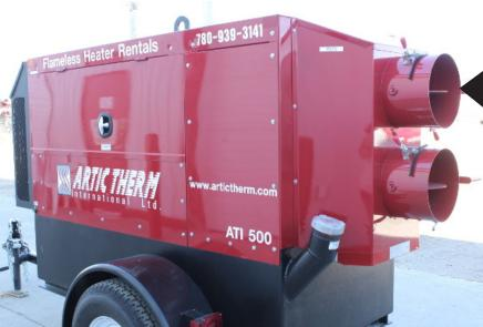
**500** 77°C / 171°F 600,000 BTU 5,000 CFM 4.2 Imp Gal/ 19 L per hr **900** 83°C / 180°F 1,200,000 BTU 7,200 CFM 7.6 Imp Gal/ 33 L per hr
